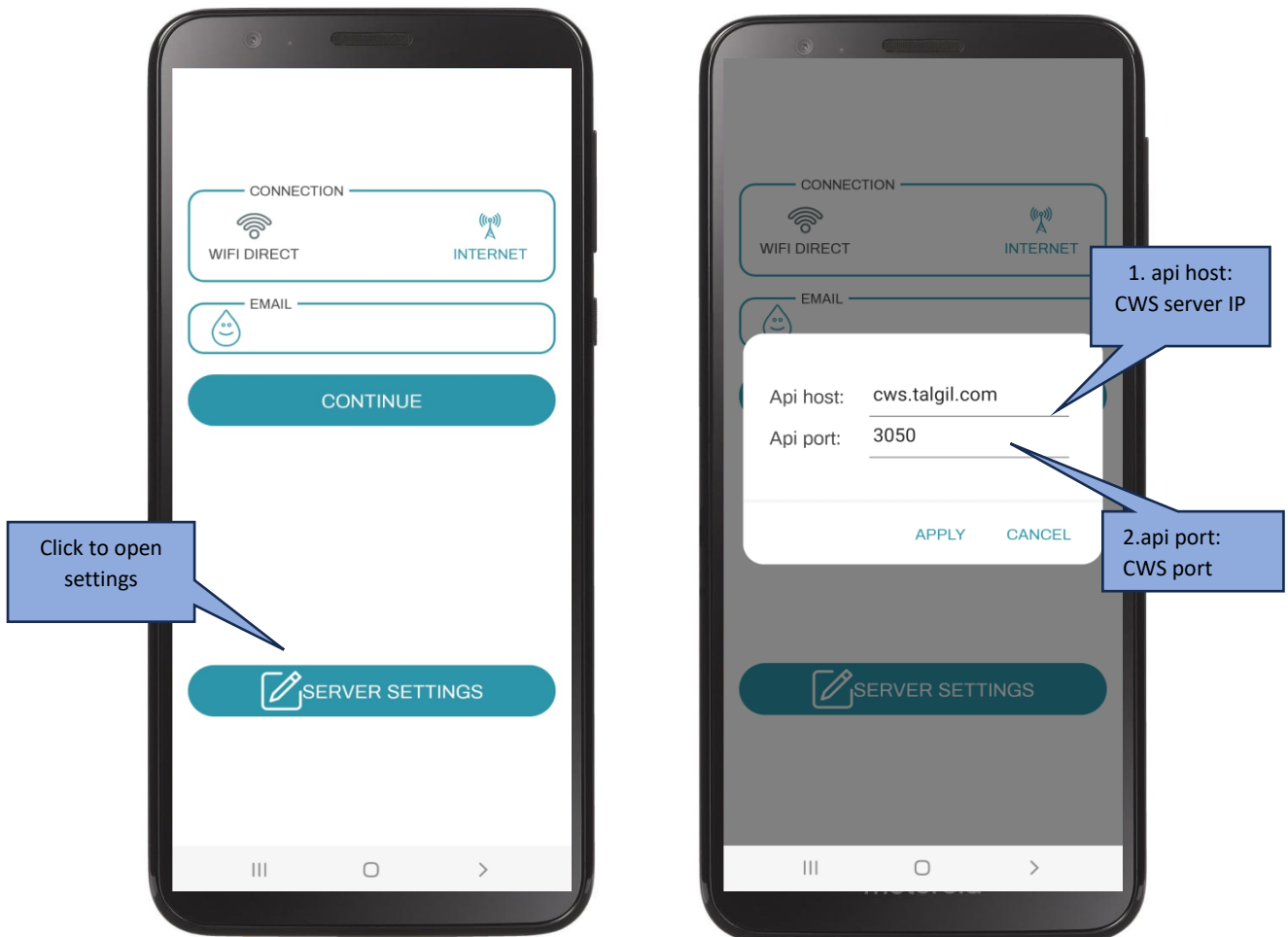
Fig 13 – configuring user side server IP/port details
