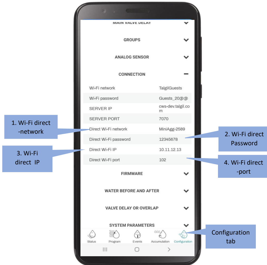
Fig 9 – configuring Wi-Fi Direct connection details
