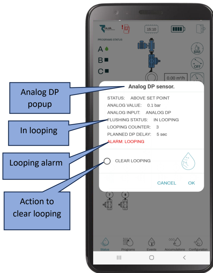
Fig 50 - analog DP in looping state
