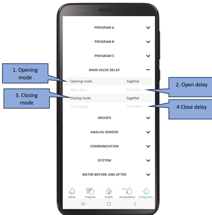
Fig 65 – main valve delay section
