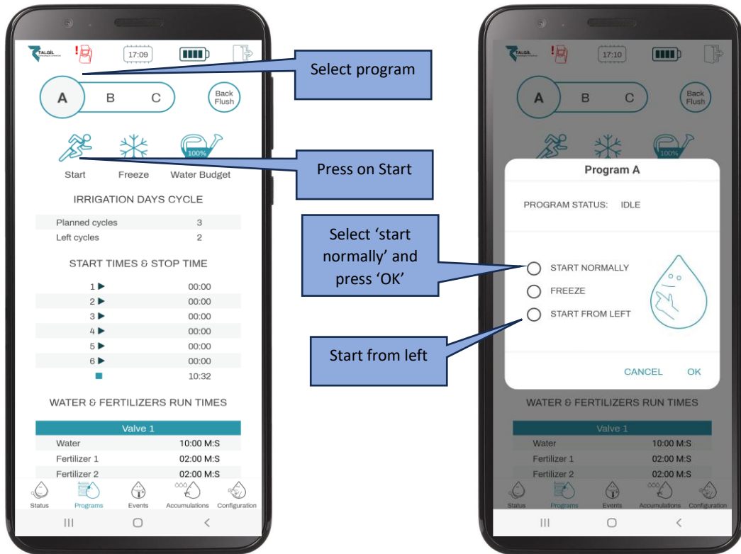
Fig 36 – starting program manually from program tab
