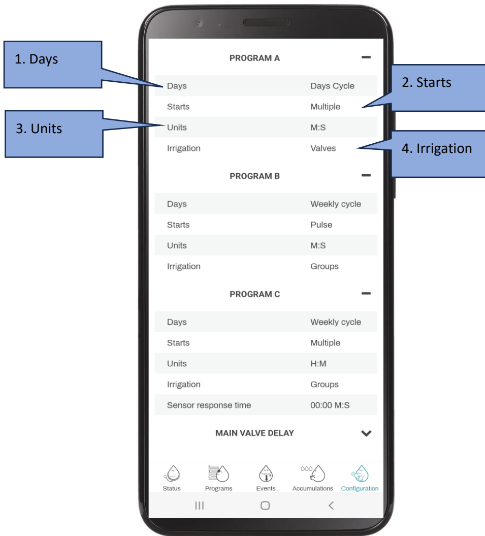
Fig 27 – program configuration details
