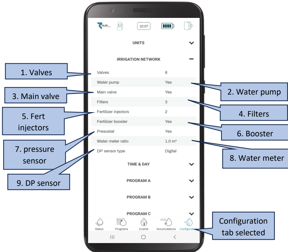
Fig 24 – irrigation network details
