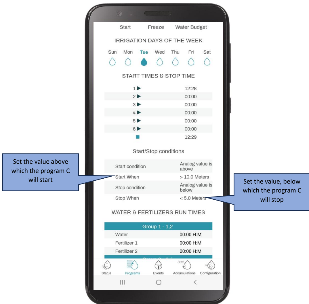
Fig 60 – Analog sensors start/stop configuration
