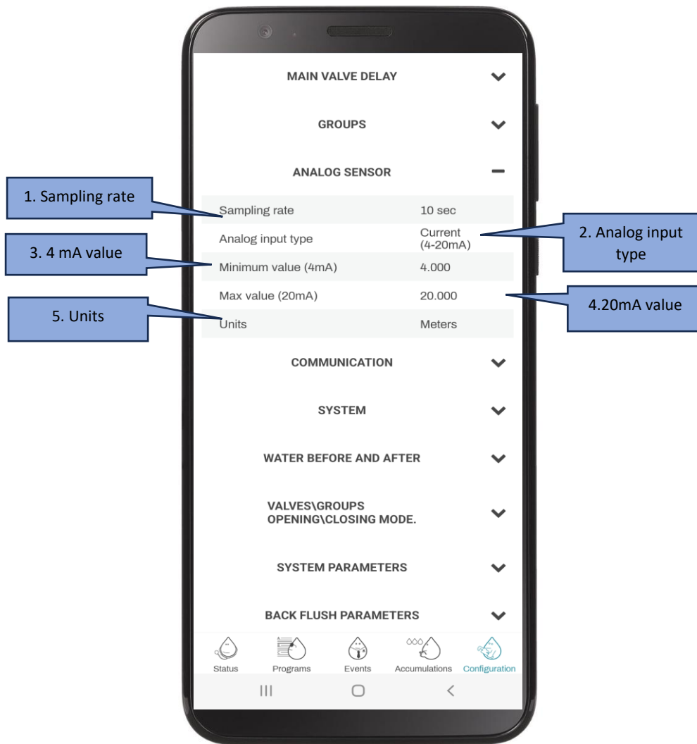
Fig 57 – Analog sensor configuration details
