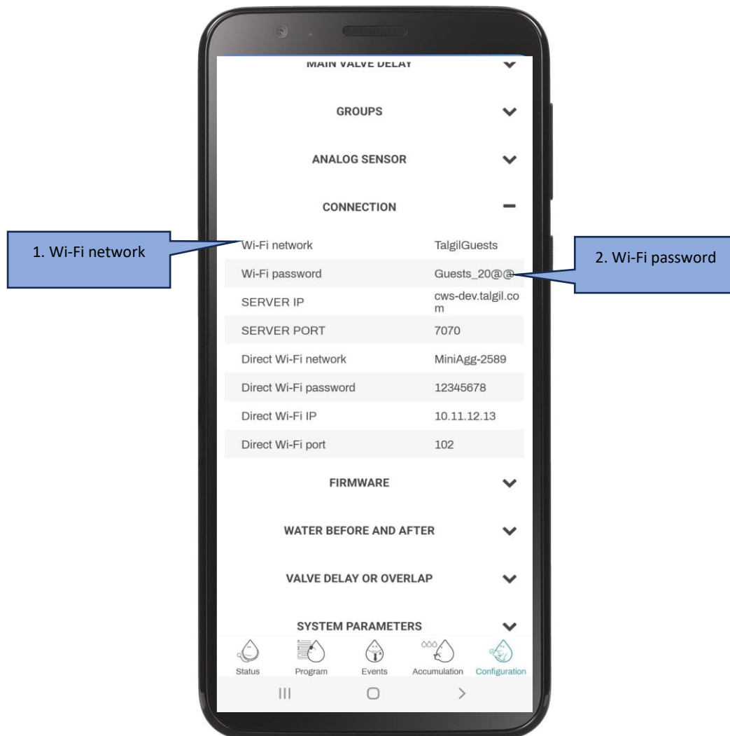
Fig 11 – configuring Wi-Fi modem details
