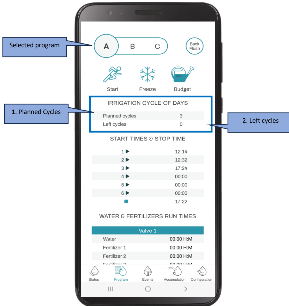
Fig 29 – Irrigation by cycle details for program A
