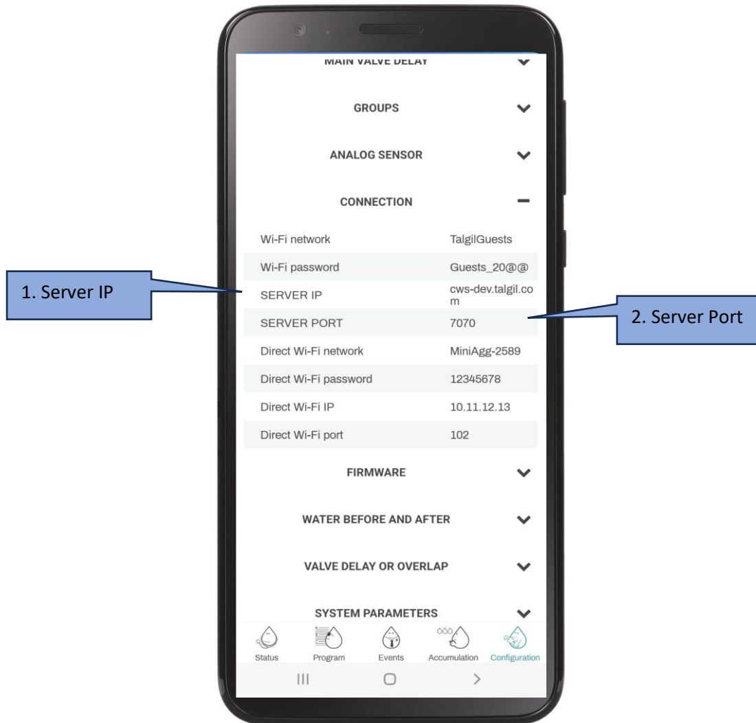
Fig 12 – configuring controller side server IP/port details
