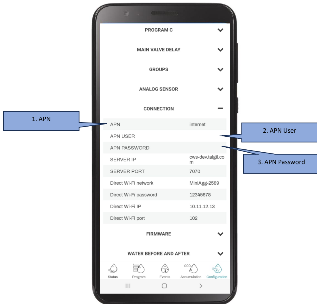
Fig 10 – configuring APN connection details
