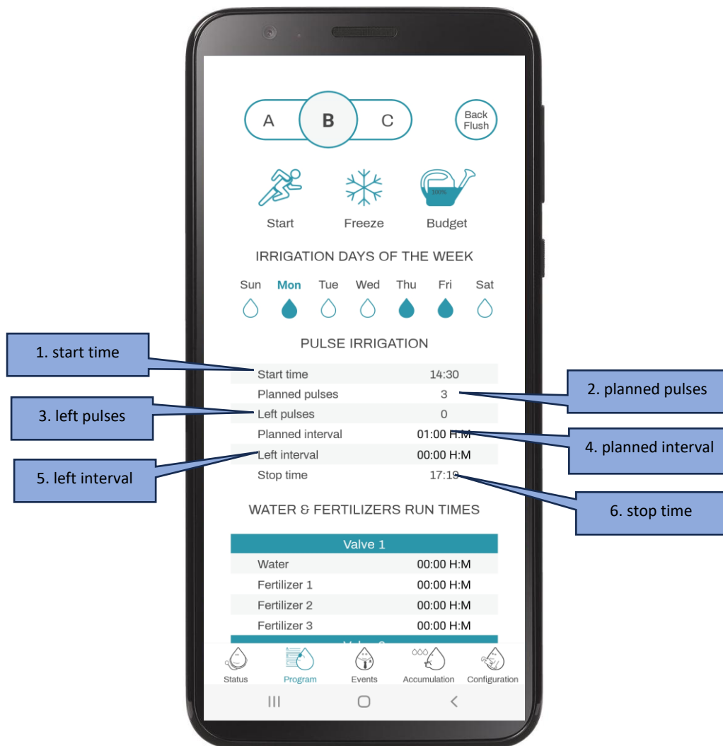
Fig 32 – configuring pulse irrigation details for program B
