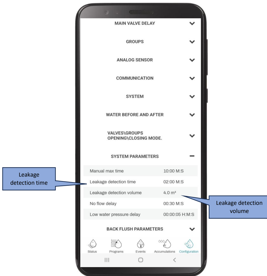
Fig 53 – leakage detection parameters
