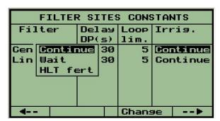
**Looping limit** – defines the number of consecutive flushing cycles caused by the DP indication, after which an "Endless looping" problem is declared.
