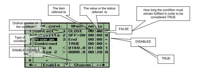
Whenever a combined condition is being defined an auxiliary screen appears in which the user may define the formula of the combination.
