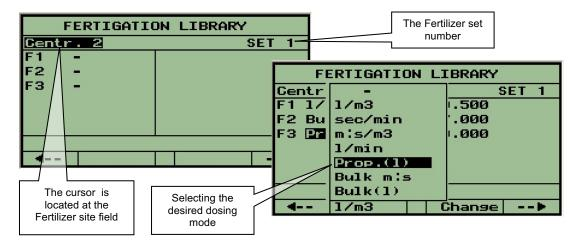
The picture at the right shows how irrigation programs can use the Fertilizer Set. The user specifies the desired Set number in the fertilizer dosage screen; the predefined set will immediately pop up and save the labor of repeatedly defining the same dosages whenever the same recipe is needed.
