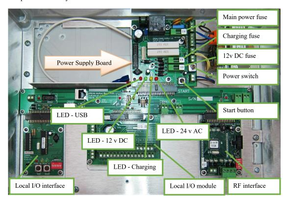
When the **Power Switch** is off, only the yellow LED should keep on lighting, indicating that the charging of the backup battery continues.
