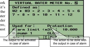
If the result is not zero, it indicates leakage of the network. However, since there may be some delay between the sensing of the water meters feeding the system and the sensing of the consumer water meters, we may get temporary nonzero values, which may create false alarm situations. Alarm limit must be set so that only when the limit is exceeded, the network protection will start to be considered, and only if it remains out of the limit for 4 minutes, the alarm will be fired.
