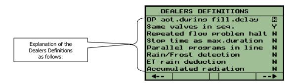
**DP** act. during fill. delay – this parameter defines whether during filling delay the DP contact will be referred to or ignored.
