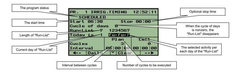
The days of operation can be specified either by defining a nonzero cycle of days or by setting up a "Run-List". The length of the "Run-List" can go up to 16 days, the user should mark each day the desired activity of the specific day: (f) indicates fertigation, (w) indicates water only (-) indicates no activity and the symbol (s) indicates single time activation (but including both irrigation and fertilization).
