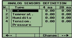
The analog sensors can be used for conditioning the system's operation and can be logged for analyzing the system's operation.
