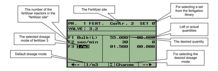
Locate the cursor at the dosage mode field next to the desired fertilizer number. Select the desired dosage mode either by using function key N<sub>2</sub> for selecting the default mode or function key No. 3 for opening all the dosing options. Define the desired fertilizer quantity or desired proportion.
