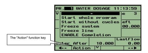
**ENABLE COMPLETION** – is an option that can be activated per each program individually. Once activated the option remains active until giving the opposite command. A program with enabled completion feature, will check at the end of its irrigation whether some of the included valves have uncompleted dosage (probably because of some malfunctions). The system will try to complete those leftovers.
