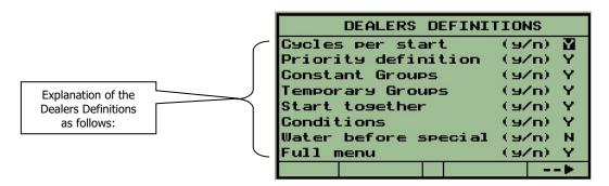
Cycles per start – enable irrigation in cycles, which means repeating the irrigation a specified number of times.
