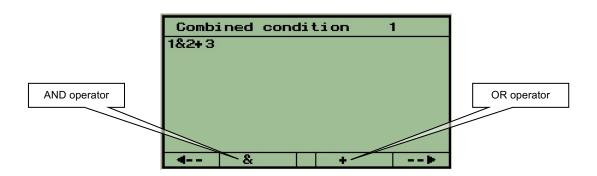
The formula 1&2+3 should be interpreted as 1 & (2+3) which means that in order for the combined condition to become TRUE, condition No. 1 must be TRUE, AND conditions No. 2 OR No. 3 must be TRUE.
