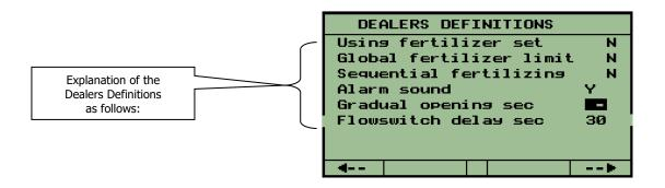
Using fertilizer sets – enable using fertilizer sets. The fertilizer sets are predefined formulas of fertilization to be used by the irrigation programs. See the subject **FERTILIZER SETS LIBRARY** in the submenu of **PARAMETERS**.
