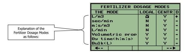
In the screen above, we can define which of the fertilizer dosage modes will be revealed to the user. There can be a different definition for local and for central fertilization. The column marked "D" defines which mode will be the default mode.
