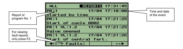
When the cursor is placed at the word REPORTS as shown above, pushing **F2="Faults"** will display only the fault reports.
