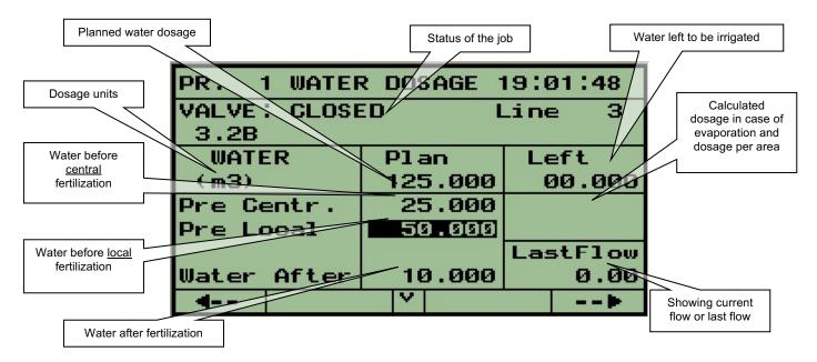
There is an option to define a special dosage of "water before" for Local fertilizer №1 to make it different from the others. This option must be enabled through the **DEALERS DEFINITION**.
