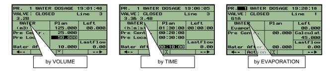
Notice that when irrigating by evaporation (or by m3/area) there is no planned value to be inserted but there is a calculated value. For detailed explanation of dosage by evaporation and dosage by volume per area see appendix "A" of special dosage modes.
