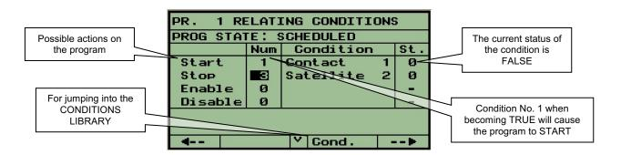
By specifying the ordinal number of the desired condition in the row of the desired action we create a relation that will cause the action to be executed when the condition becomes TRUE.
