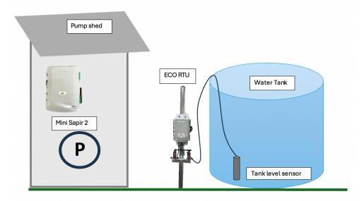
By adding in 1 **ECO RTU** to the system as well as monitoring the Tank levels, the **Mini Sapir2** can be in the pump shed on site and start your pump to fill the tank based on the readings you are receiving from the tank level sensor which is connected to the ECO RTU. Water will start filling when the tank is low and will stop filling when the tank gets full.
