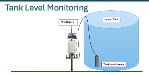
Using the **Mini Sapir2** and a **tank level sensor** we are now able to offer a more cost-effective method to monitor tank levels and give you readings of what the levels are at, you are also able to format that information into graphs for easy viewing.
