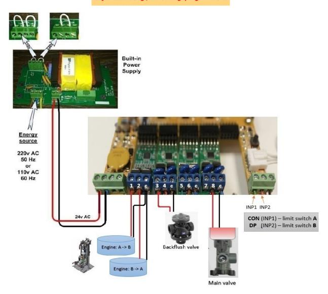
1. The controller will be powered with built-in PS 24V AC outputs.
