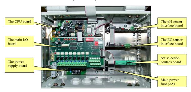
The following picture shows the main I/O board explaining the function of its main parts.
