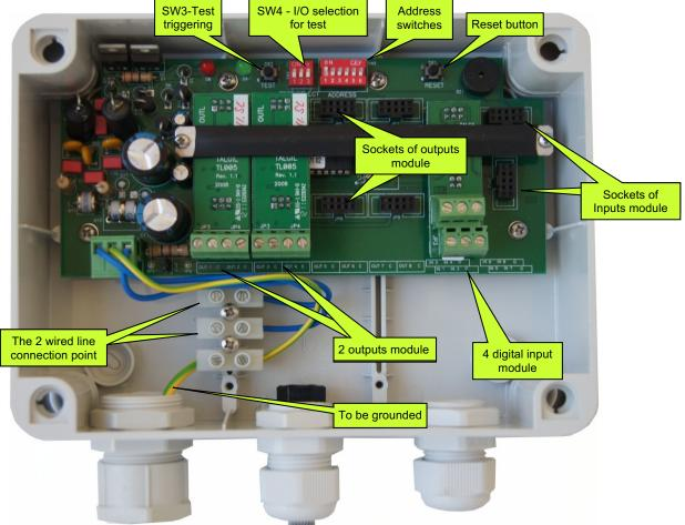
The system can handle analog inputs as well. There are "plug in" modules of 2 analog inputs that can be used in place of each module of 4 digital inputs, using the same sockets. Therefore, each analog inputs module reduces the number of left digital inputs of that RTU by 4.
