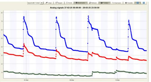
The graph above is extracted from the **EnviroPro** probe which is a 80cm length sensor, which has the ability to measure every 10cm of soil depth. Above you can see the 20cm, 30cm and 40cm reporting moisture back to the Dream Controller via G5 radio RTU.
