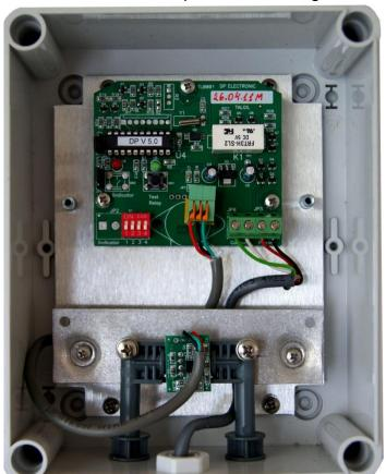
Black command tube to **low** pressure point Red command tube to the **high** pressure point
